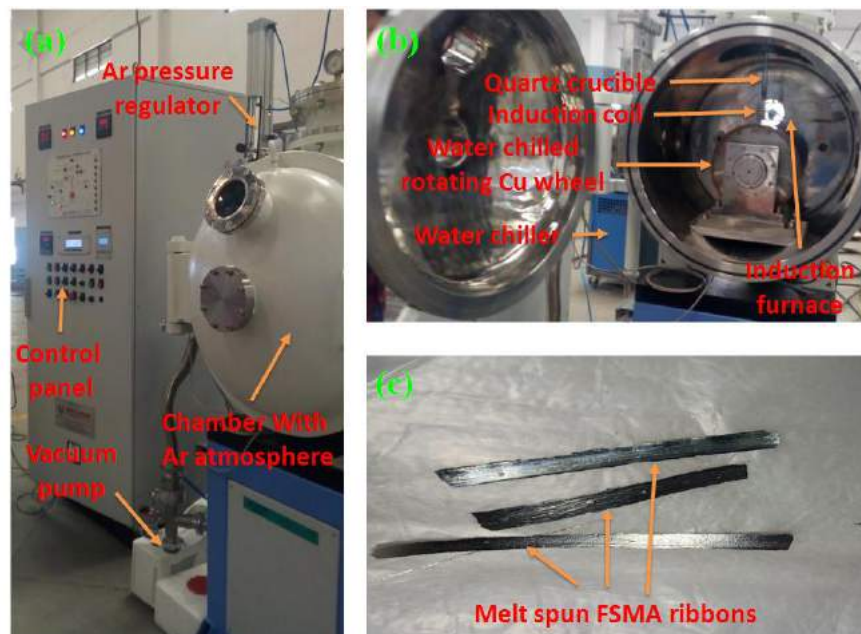
Figure 2.7 (b): RF Induction furnace used for Finemet Sample preparation
