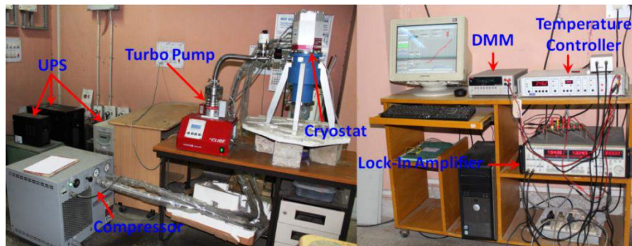
Figure 2.15: The picture of the experimental setup for measuring low temperature resistivity.
